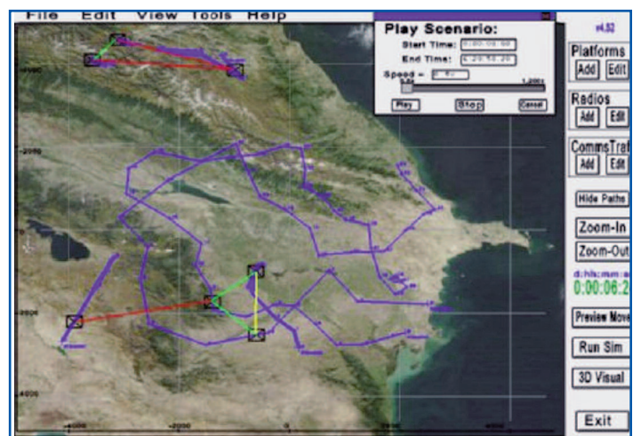
The Scenario Entry view is the basic tool to load the detailed mission plan, including terrain and mission equipment into COMPOSER.
