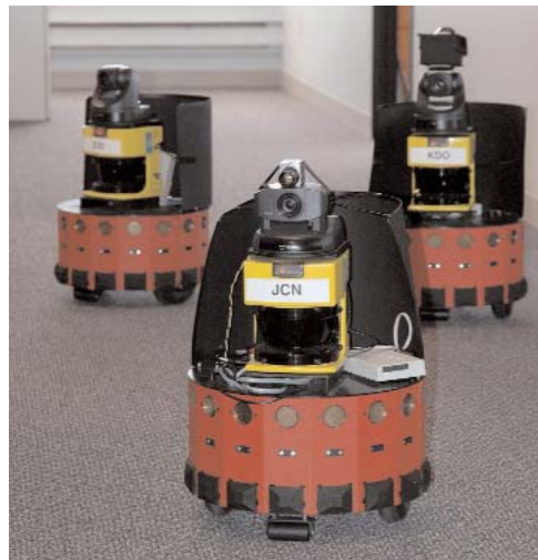
A team of robots embark on a role-based team mission from ATL's robotics laboratory. Each robot has a specific role as well as an understanding of the roles of its teammates.
